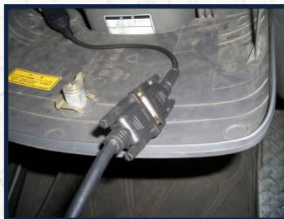
2.Connect the diagnostic cable
