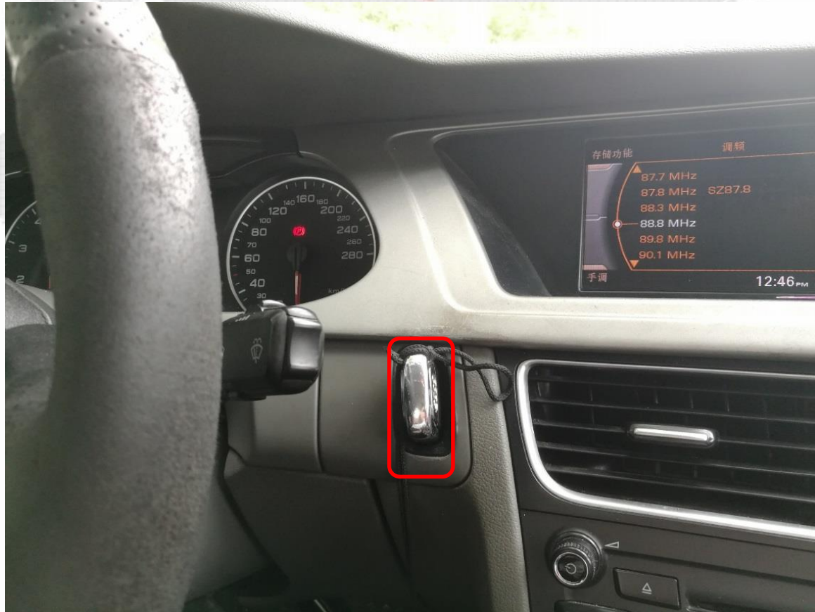
1. The original car smart card is inserted into the card slot and lit up the Dashboard
