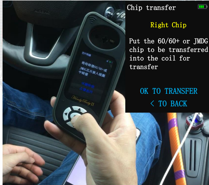
3.6. Put the 60/60+ chip to be transferred into the identification antenna, OK button to transfer
