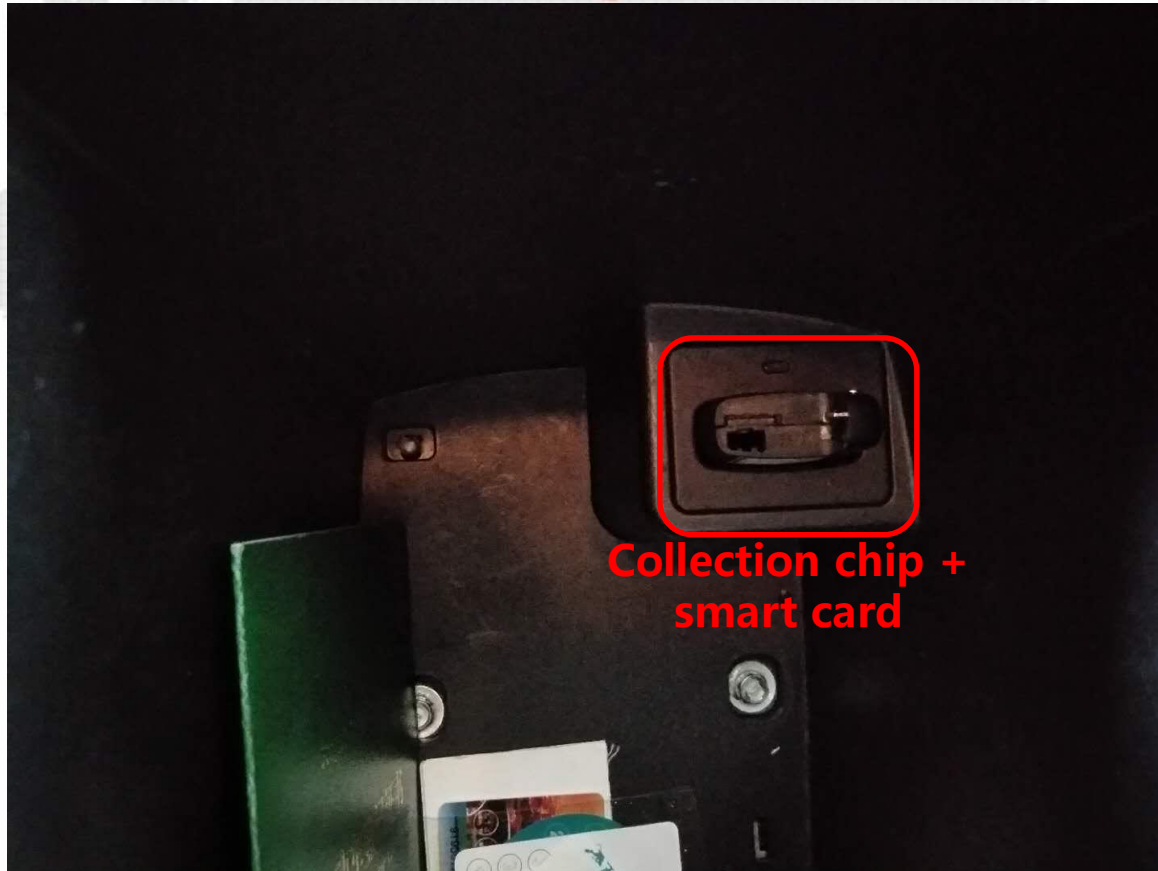
5. the original smart card and C-JMD6 together put into slot and light meter
