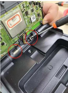
4, Please remove the plastic pin socket from screen cable with sharp piler like picture show, for remove whole screen and cable from machine xp005L,
