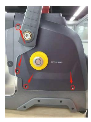
${\bf 2}$  , Take out those screws and disconnect cables as picture show , for remove back case from screen
