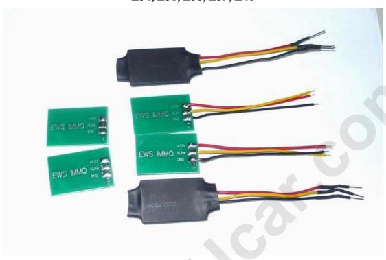
This device can emulate BMW EWS 2 and EWS 3.2 immobilizer (EWS module) in cases when original system restore is impossible (faulty EWS, lost or damaged transponders, continuous problems with rolling codes etc.).
