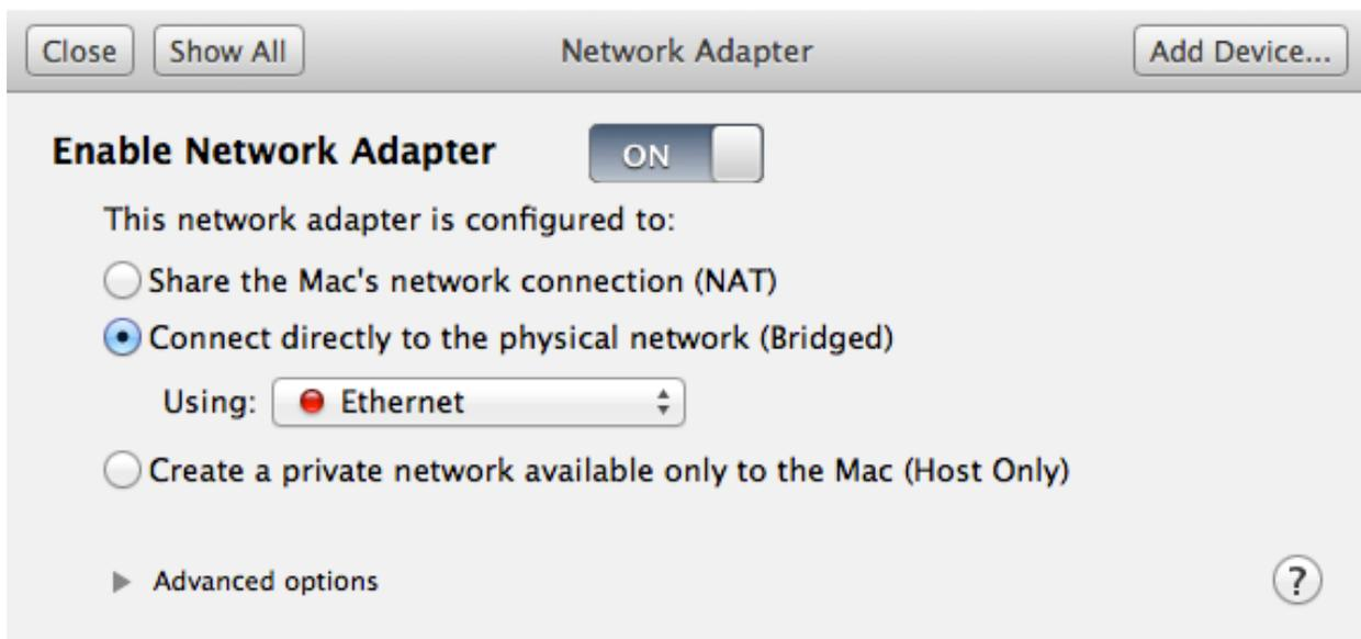
*Note: at the time this screenshot was captured, the Ethernet wire was not connected to the car, hence it is shows a red circle in front of the title "Ethernet". Once connected to the car (or any active ethernet wire), the circle will be green.*
