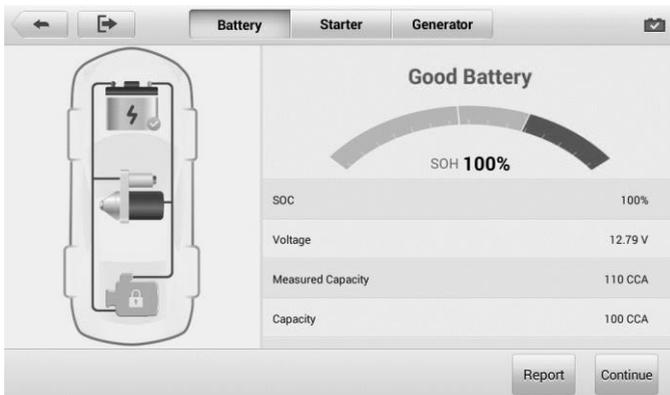
**Figure 6-7 Sample Battery Test Results Screen**
