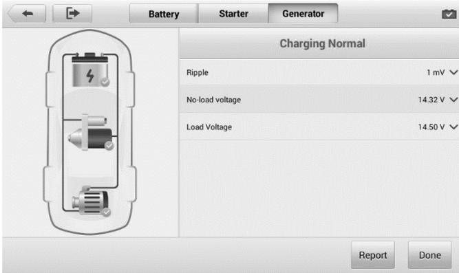
**Figure 6-10 Sample Generator Test Results Screen**
