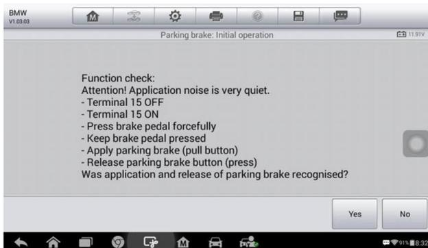
**Figure 5-7 Sample Parking brake: Initial operation Screen 1**
