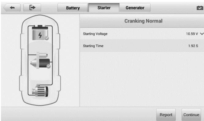
**Figure 6-9 Sample Starter Test Results Screen**
