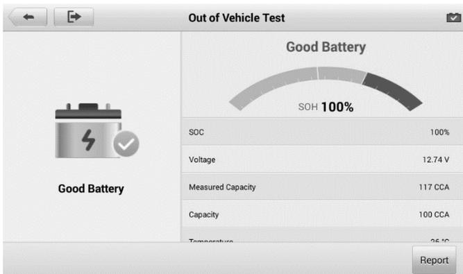
**Figure 6-12 Sample Out of Vehicle Test Results Screen**
