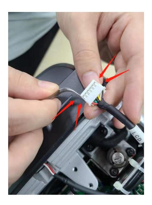
Remark: Please take a photo for that pin socket before you remove it, all pin should be in the exact same position like before when you put it back
