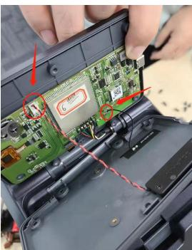
3, Use the flat head screwdriver to push out the mount which use for fix the screen like picture show, for remove screen from the back case of machine xp005L
