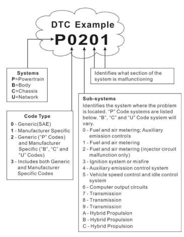
P0201 - Injector circuit malfunction, Cylinder 1
