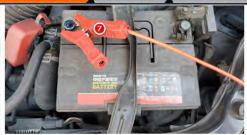
Step 6: Select Read Immo Data menu to read immo data and save it to the device(Select the saved data to generat e the start key,Then proceed to key programming), It is recommended to use the Key SIM to generate the start key; Step 7: Remove all the connections between the TOYOTA-2 cable and the vehicle, connect the positive cable of the vehicle to the positive terminal of the battery, Select the saved Immo data to generate the start key, Then proceed t o key programming;
