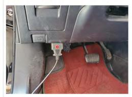
Step 3: Remove the lower shell of the vehicle ignition switch lock, pull out the plug of the ignition switch lock, plug of the ignition switch lock plug into NO.5;
