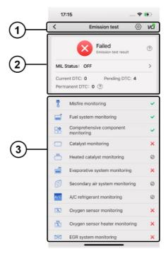
Figure 4-8 Emissions Test Screen
