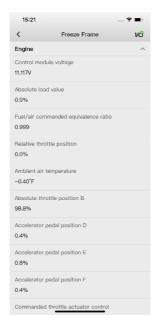
Figure 4-11 Freeze Frame Screen
